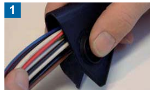
1 Push tool over cables
